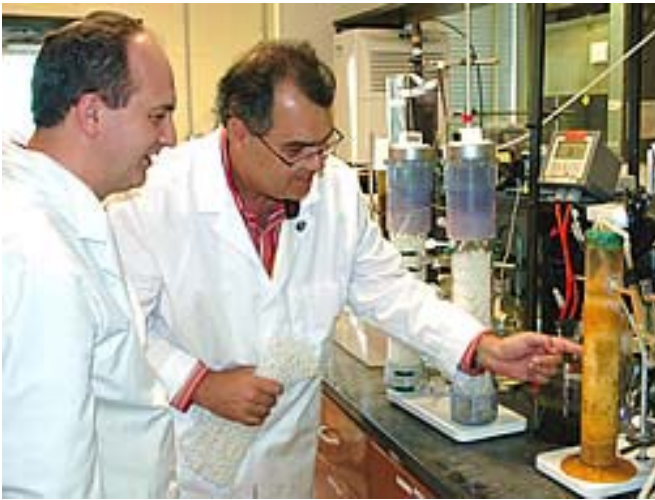
Soil scientists Ariel Szogi (left) and Matias Vanotti examine a packed-bed bench reactor containing the anammox bacteria immobilized in polymer gel beads. Image courtesy Matias Vanotti.
